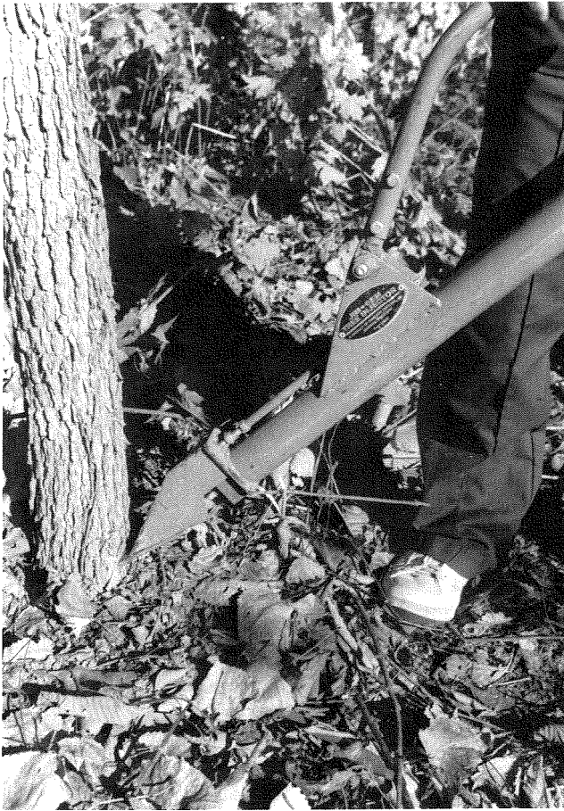
Figure 9.-Tubular injectors are jabbed into the base of the tree at a 1 -inch spacing around the tree. This equipment has a long history of use in forestry. (Harvey Holt)
