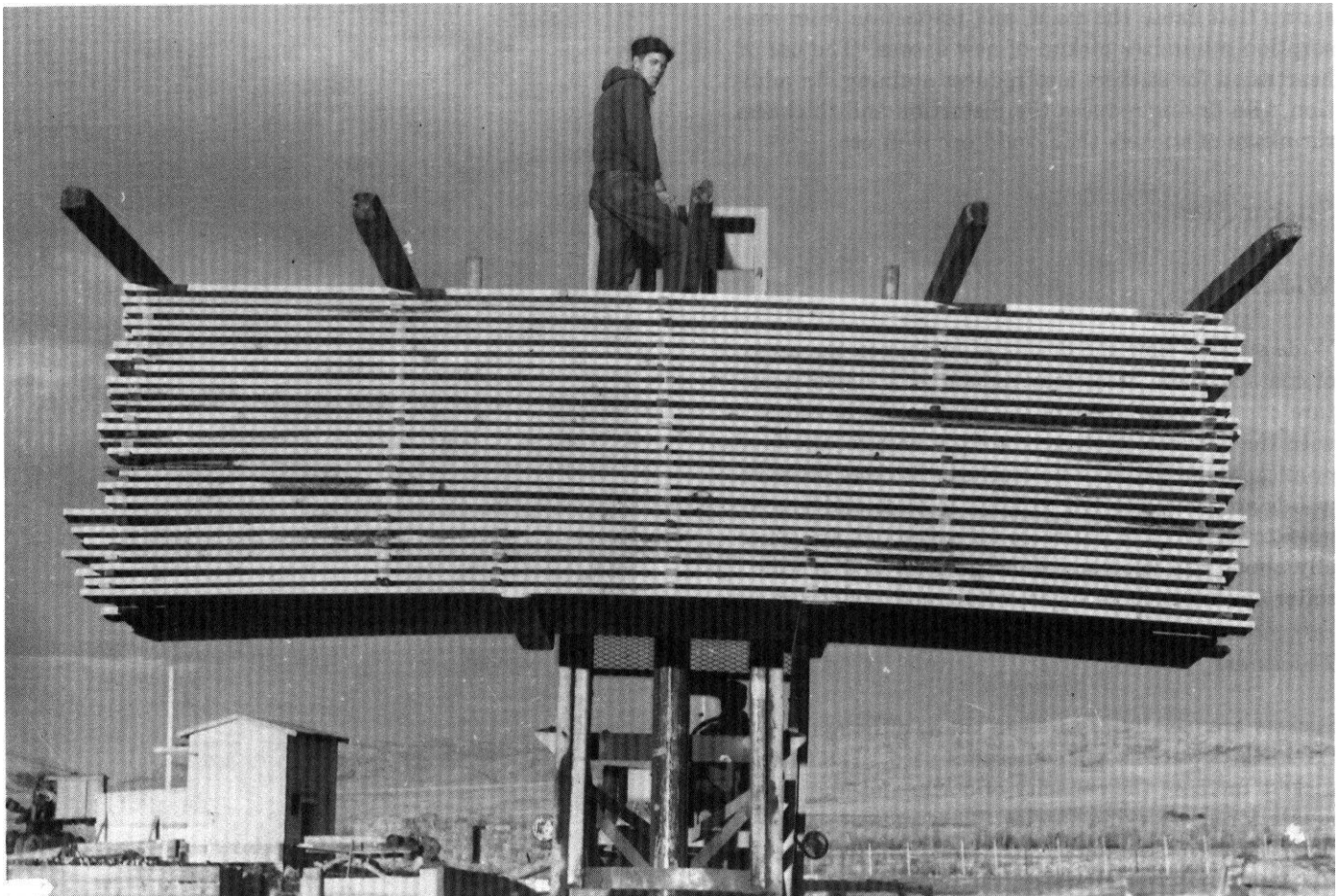
Figure 5-6—Package of lumber raised by forklift truck. Short tiers of stickers above point of contact with forks reduce sag in the lower courses of lumber and help
