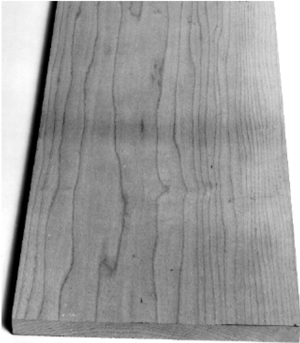
Figure 12–17. Sticker stain in sapwood of sugar maple after planing.
