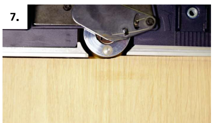
7. Use the planing machine to adapt the components to the spatial situation.
