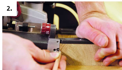
2. Transfer the centre of the milling to the workpiece.
