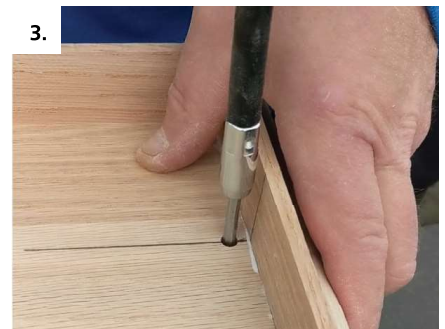
3. Glue and assemble nosing to tread with Clamex P-14 by engaging cam lock
