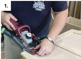
1. Lay out and machine P-System slots for top edge of front panel
